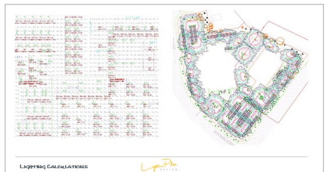
This is an example of a complete floor lighting levels and a parking area.
